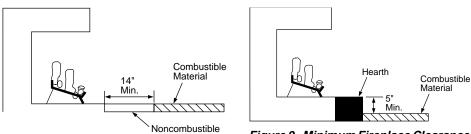
Figure 8 - Minimum Fireplace Clearances If Installed at Floor Level
